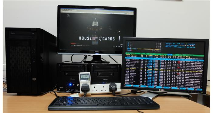
Fig. 1: Our video playback testbed. The black Shuttle systems (centre) were used for the playback experiments, and are connected to the Kill-A-Watt/MoteWatt power meter (centre-left, just above the keyboard). The mini-tower on the left is the experiment-controller, not part of the system being measured. The energy consumption of the display units was not measured: one shows the video being played back (centre), the other shows part of the measurement system (right).
